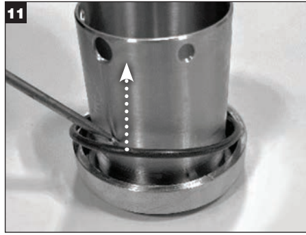
11 Remove the O-Ring (W) from the sleeve O-Ring groove and discard.
