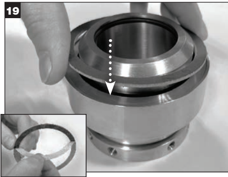
Peel off the adhesive backing from the gland gasket and install in the gland gasket recess.
